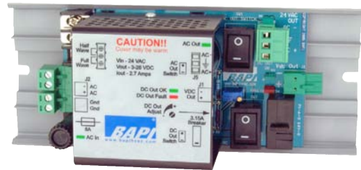
VC2700-STM - Voltage Converter with included 8" piece of 2.75" Snaptrack
