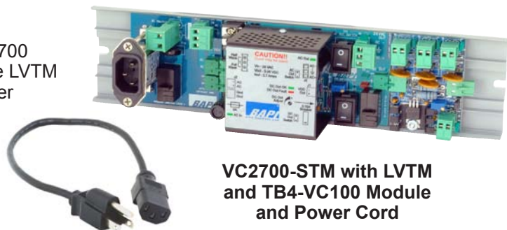
VC2700-STM - Voltage Converter with included 8" piece of 2.75" Snaptrack
