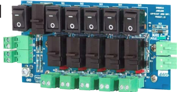
PDM - Power Distribution Module BA/PDM-5-B
